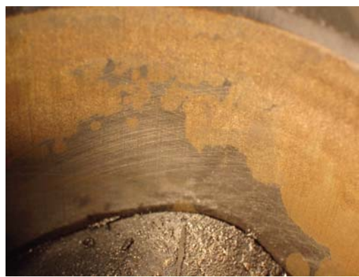
Figures 5 and 6: Corrosion inside the National Museum Landrover cylinders
