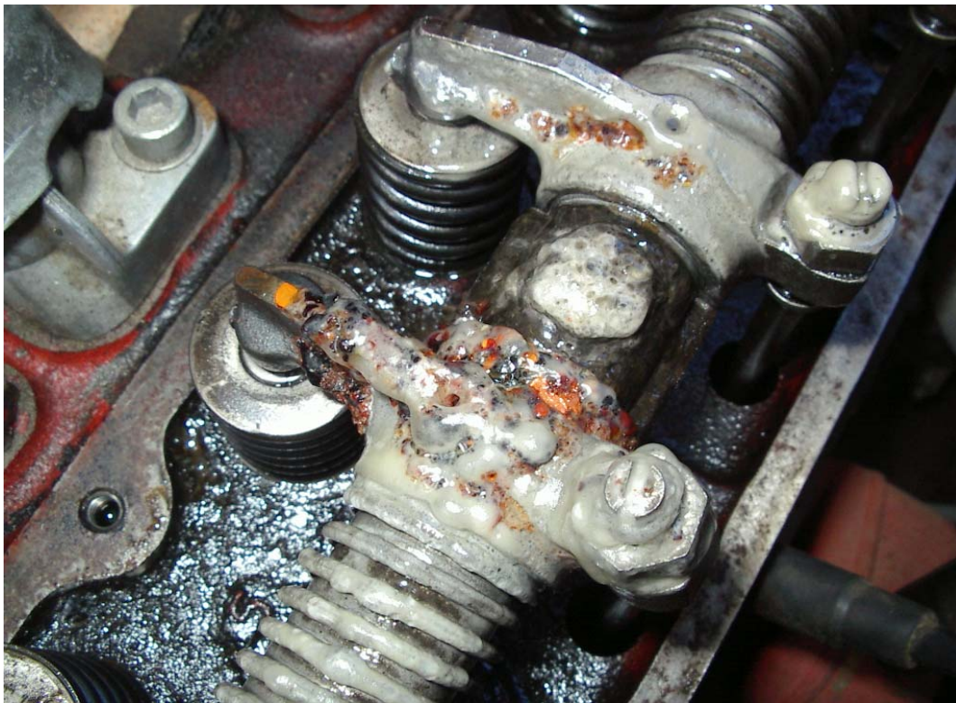
Figure 4: Corrosive gel on Volvo rocker covers after an engine has been run without coming up to temperature.
