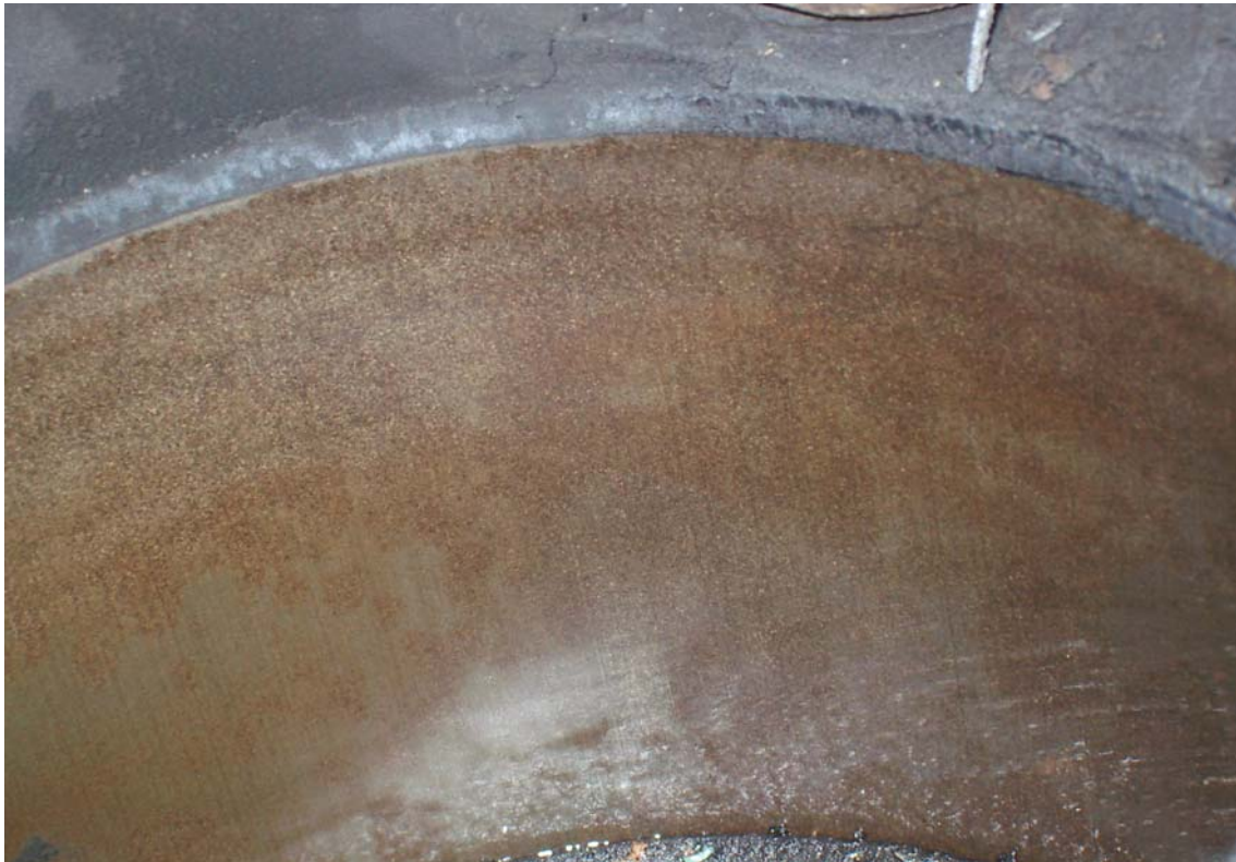
Figure 3: Rust on the inside of a cylinder in an engine from the National Museum collection.
