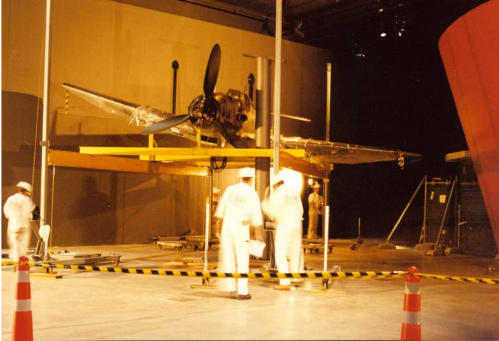
Figure 5. Aircraft halfway up. Staff checking measurements and levels to confirm correct orientation before proceeding further.
