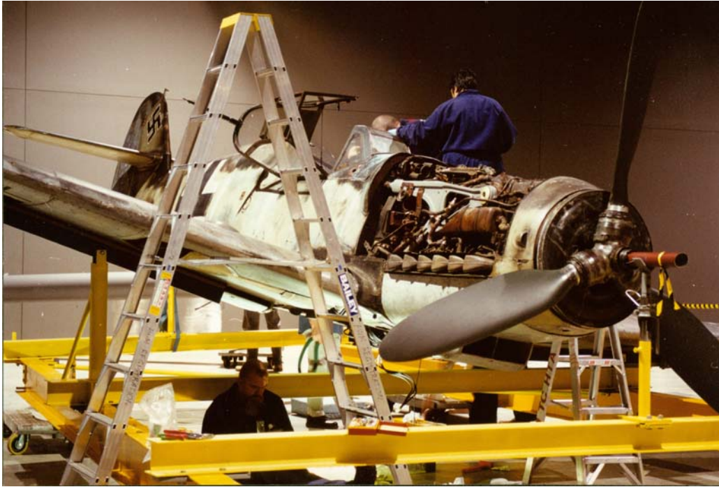
Figure 1. Assembly of the lifting frame underneath the aircraft fuselage. The aircraft is in its display orientation. The frame incorporates standard lifting beams of various sizes bolted together with fish plates, as well as tailored wing spar supports, prop spindle support and tail support.
