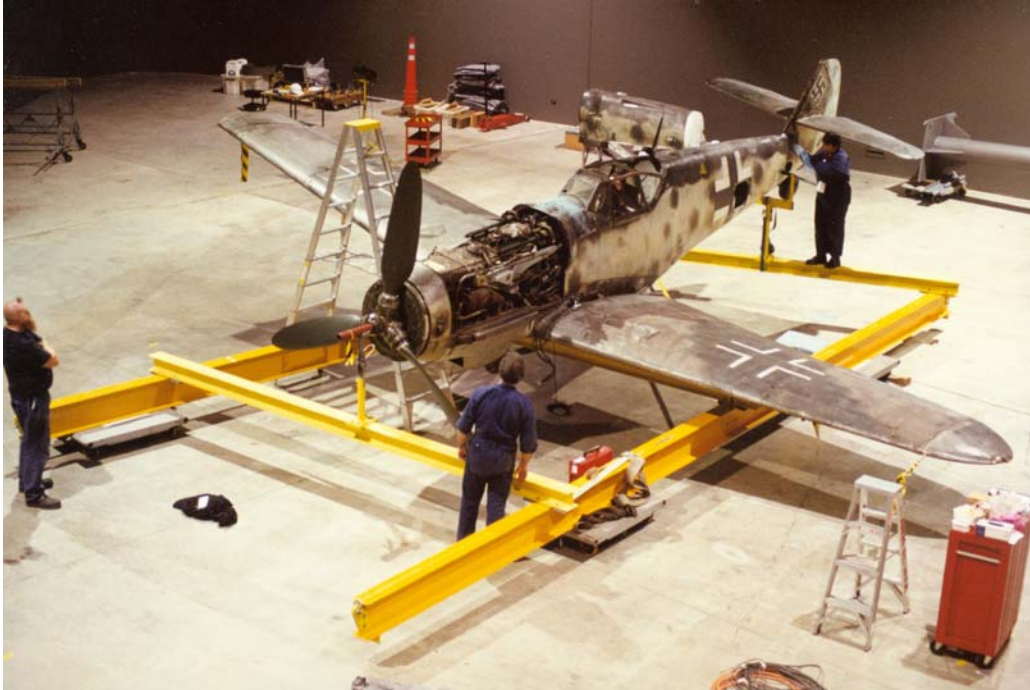
Figure 2. Wide shot showing the layout before site positioning. Note tail support which uses the standard lifting position on the fuselage.
