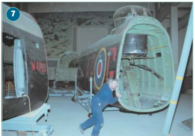
The fuselage is only one of over twenty major sections of the Lancaster: it is dismantled at the transport joints and moved away from the rest of the aircraft.
