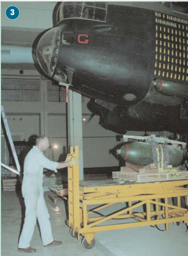
The original reason for “G for George”, the bombload, is removed from the bomb bay.
