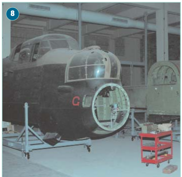
Now separated from the rest of the fuselage, the nose section sits on trolleys before its removal from the building.
