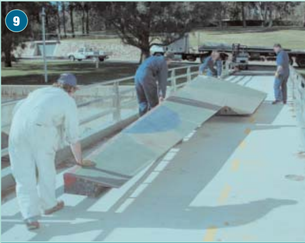
The trailing edge section of one of the wings is carried towards a waiting truck.
