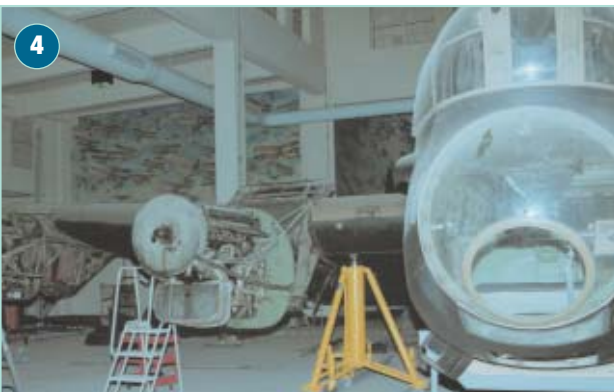
The Merlin engines are taken off in pairs; the outer pair is removed before the inner pair. Here they have been stripped and await removal.
