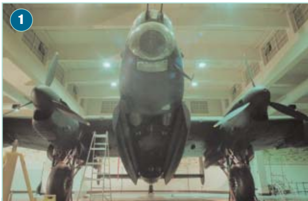
After removal of the undercarriage, “G for George” is ready to be lowered on hydraulic jacks for disassembly.
