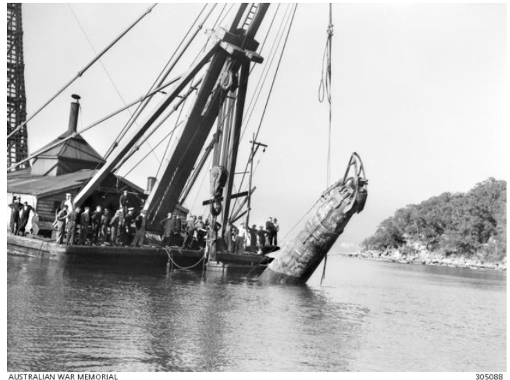
Image 5: SYDNEY, NSW. 1942-06-10. JAPANESE MIDGET SUBMARINE NO. 21 BEING RAISED BY THE BOWS FROM THE HARBOUR BY A FLOATING CRANE DURING A SALVAGE OPERATION.
